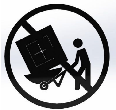
DO NOT USE A WHEELBARROW OR OTHER UNBALANCED EQUIPMENT TO MOVE UNIT
