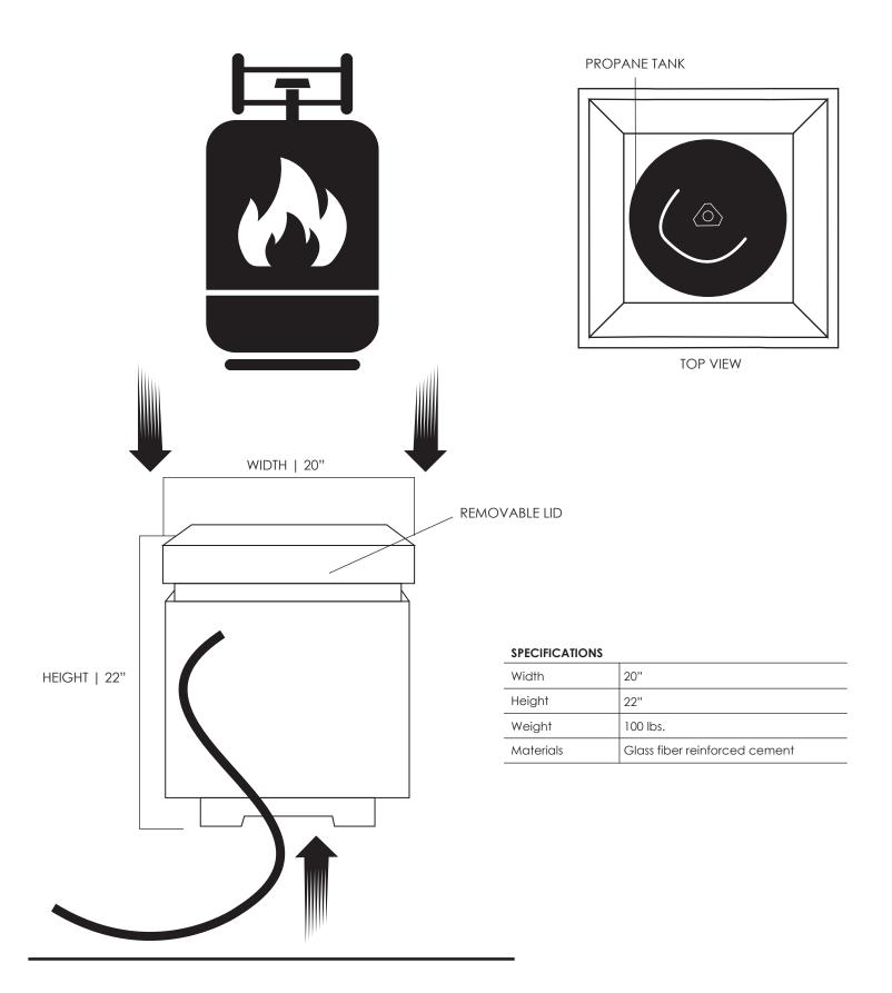
Carefully remove the lid to the enclosure. Place enclosure close enough to the fire feature to allow the hose to run freely without any kinks or pinching. Run the hose through the bottom of the enclosure. Place the propane tank (not included) into the enclosure and make sure the hose is securely connected to the propane tank. DO NOT PLACE THE PROPANE ENCLOSURE ON TOP OF THE HOSE. Place lid back on the enclosure.
